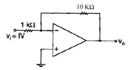
35. What is the value of output voltage for the non-inverting op-amp shown below?
