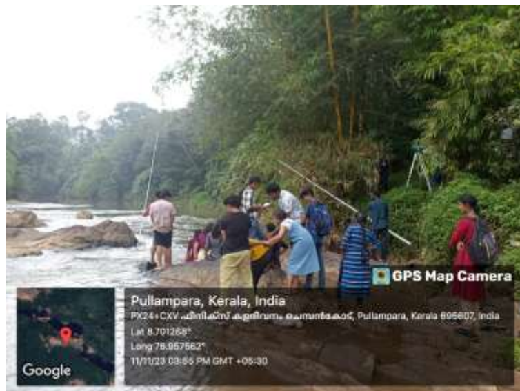
Using Dumpy level in field for river profile in the field trip by external experts
